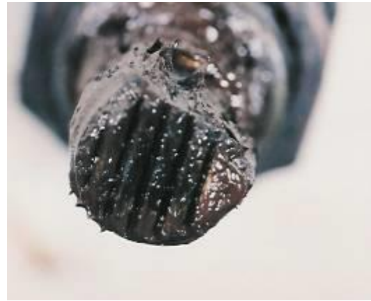
Worn/damaged Rockwell / Meritor ASA adjusting pawl
