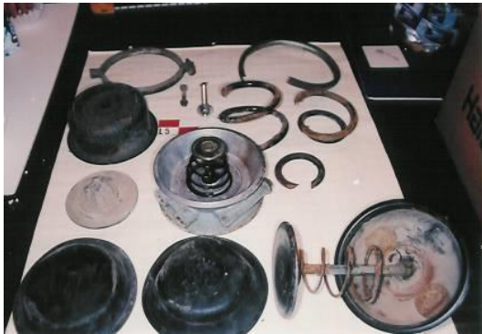
Disassembled Type 30/30 brake chamber with fractured power spring
