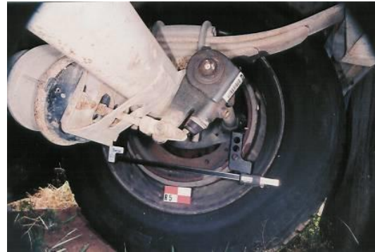
Type 30/30 Air Chamber & Meritor® ASA Note: Central™ “Wheels-On” Drum Gauge in background
